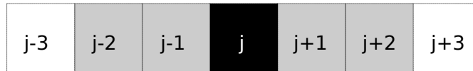
Figure 5.9.: The neighbourhood used to compute the propagated quantity in cell j (black) spans seven different cells. To compute the flux corrected value for cell j the geometric transport for cells (j - 2) \dots (j + 2) (grey) is needed.
