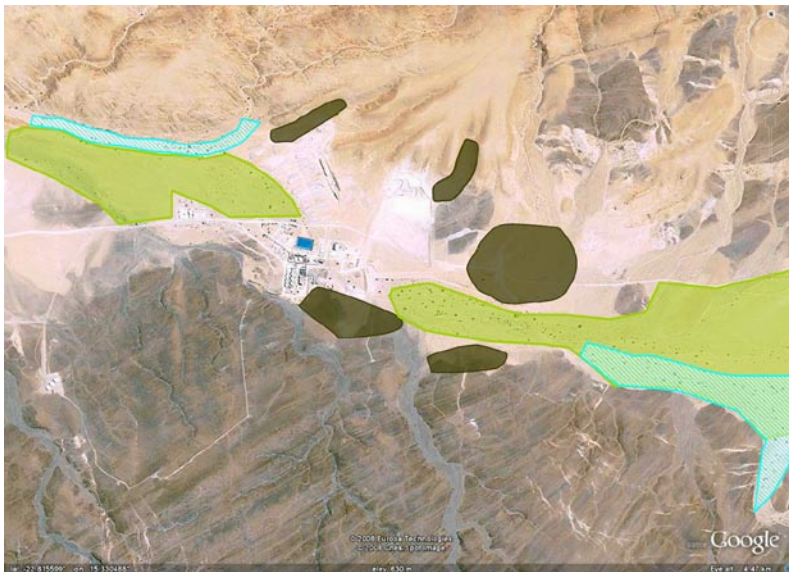
Figure 5: Areas where mitigation measures will become necessary are indicated in green. Of these, possible key seeding areas, indicated in blue, should be treated as NO GO areas. The approximate position of current stock piles, tailings facility, and mine dumps are indicated in brown.
