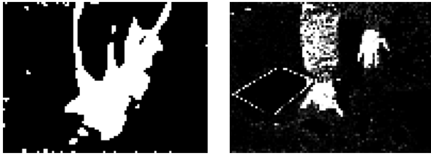
Fig. 3. Results of the motion cue (left) and colour cue (right). Usually, none of the cues alone allows perfect tracking. Only by combining several cues the robustness necessary for real world applications is reached.
