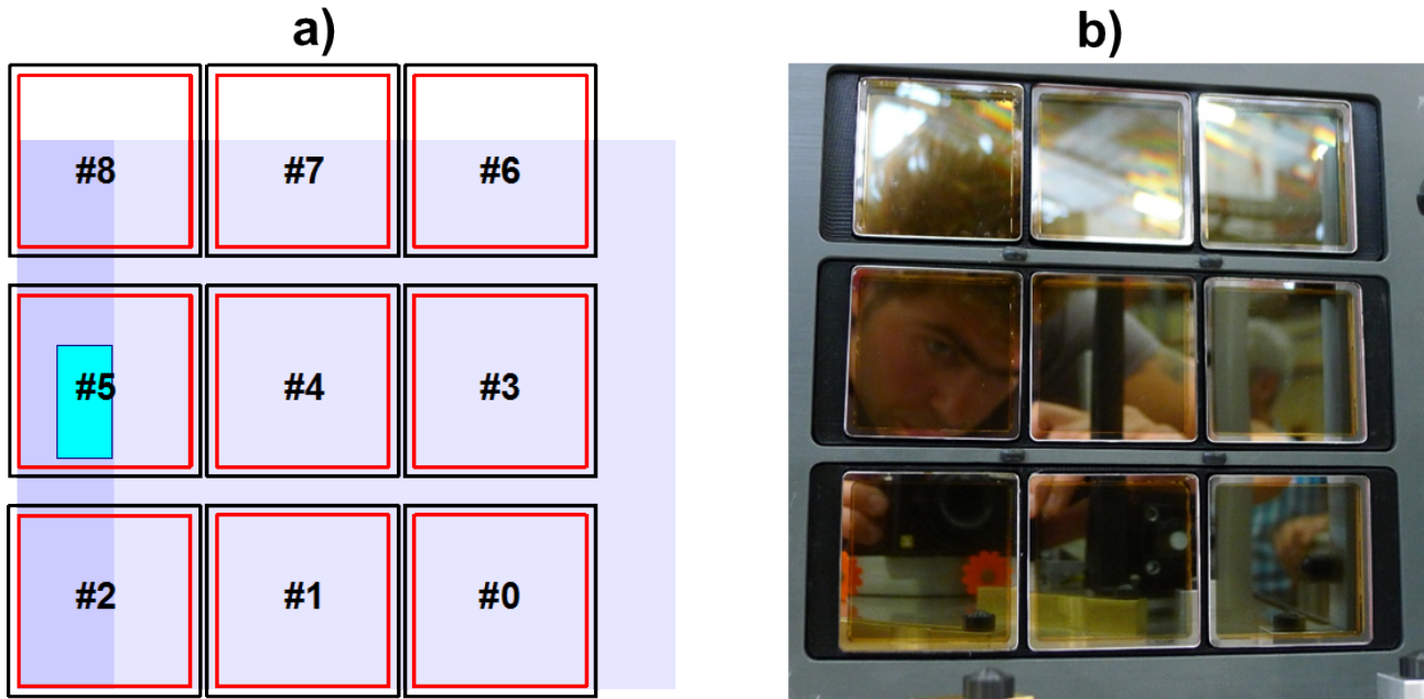
Figure 4.21: Schematic (a) and photo (b) of the MCP-PMTs arrangement on the detector plane.
