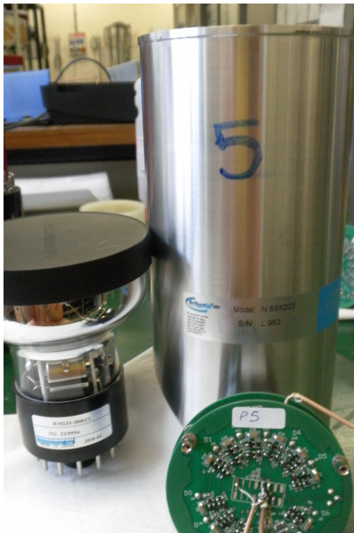
Figure 3.5 – The picture shows one of the six used LaBr 3 :Ce detectors and the attached photomultiplier. Since the LaBr 3 crystal is toxic and highly hydrophilic, they are contained within a sealed aluminum cylinder. Each detector-crystal has the dimensions of 89 mm in diameter and 203 mm in radius. The LaBr 3 :Ce detectors are used because of their excellent energy and time resolution over a energy-range between a few keV and up to 25 MeV, making them a valuable tool for \gamma -ray measurements in various experimental setups [36].
