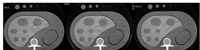
Figure 3: Images at different pitch values (120 kV, A = Pitch 3.2; B = Pitch 2.8, C = Pitch 2.2).
