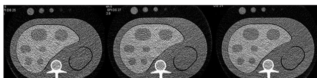
Figure 2: Images at different pitch values (100 kV, A = Pitch 3.2; B = Pitch 2.8, C = Pitch 2.2; B30 Kernel).
