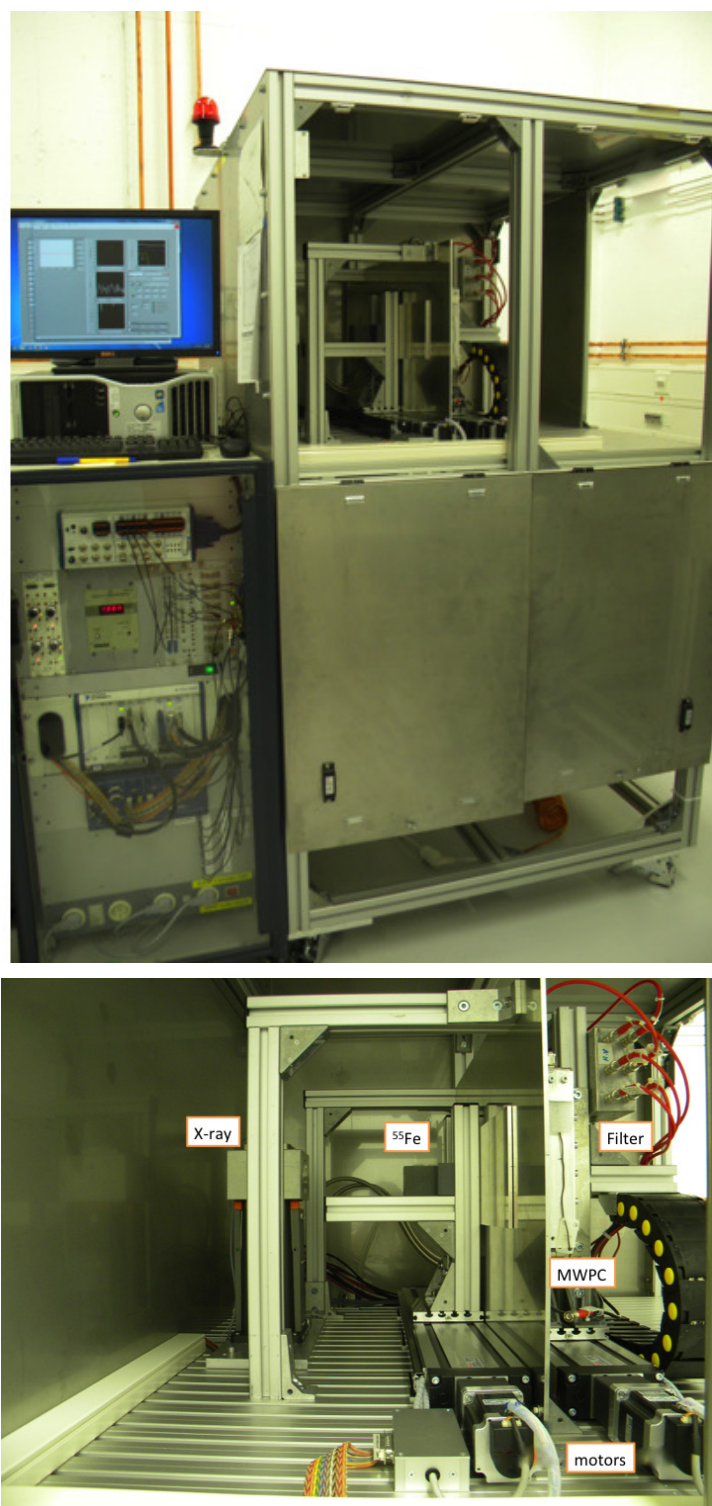
Figure 4.28: (upper) The whole box of the setup and the associated data acquisition system. (lower) Closer view of the setup components.
