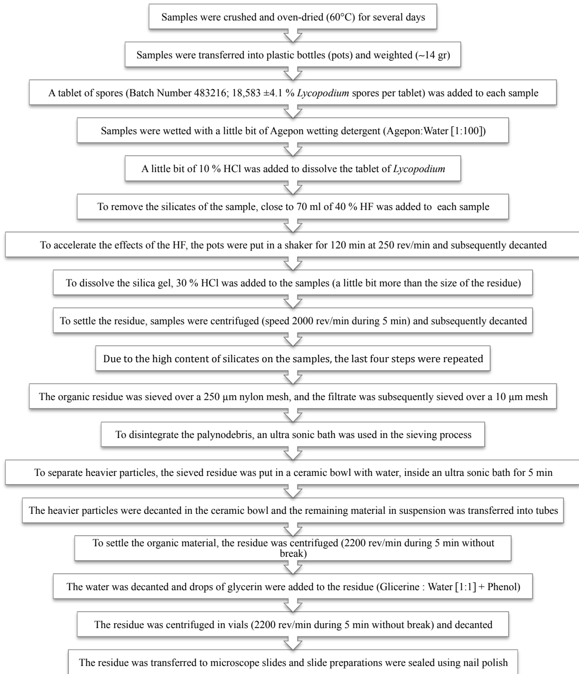
Figure 1.6 Steps of the palynological laboratory processing used for samples of Site U1356 at Utrecht University and Goethe University Frankfurt in this study. HCL was used only to dissolve the silica gel during the palynological processing due to the low content of carbonate in all processed samples.
