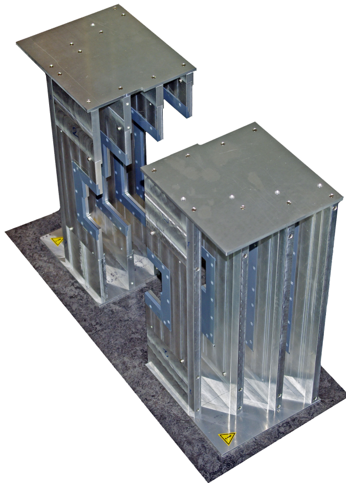
Figure E.1: The 1 : 1 mock-up of the proposed MVD geometry comprising all four MVD stations and their components. The components will be substituted with functioning elements bit by bit in the near future.
