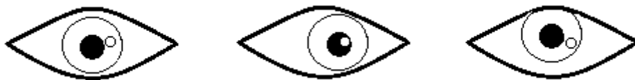
Figure 1. Schematic example of where the pupil center (black circle) and corneal reflection (little white circle) are when a person (right eye) looks straight forward, to the left and up.
