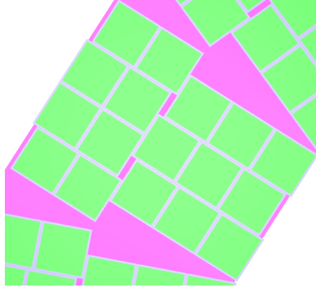
Figure 4.45: Schematic layout of the PD plane covered with MCP-PMTs when the neighbouring radial columns of MCPs are shifted with respect to each other in half of the pixel size.
