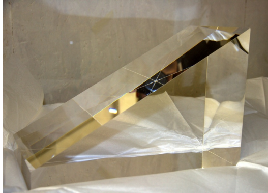
Figure 4.1: Photo of a fused silica prism used as an EV in the test beam.
