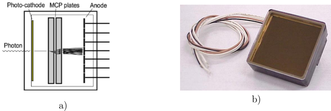
Figure 3.9: a) Working principle of the MCP-PMT. Figure from [43], modified. b) Photo of the PHOTONIS XP85012 Planacon MCP-PMT [42].
