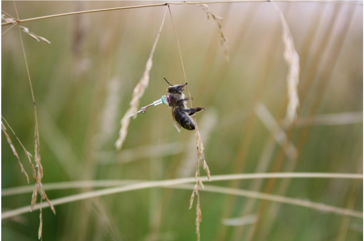
Figure 5.4. A resting bee carrying a radar transponder. The transponder had a length of 2.3 cm and a weight of approximately 20 mg. It is glued to the number tag, visible here as a small pink stripe.
