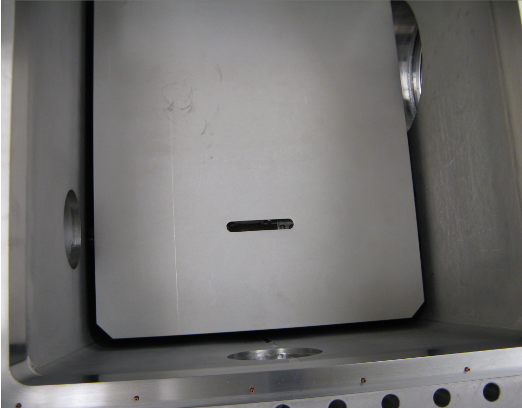
Figure A.3.: Insertion of an XY Aperture modul and the thick iron plate for the X-ray protection.
