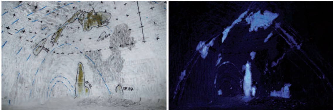
Fig. 4.3: Photo at artificial light (left) and ultraviolet light (right) of drilling station 1.2 in Crosscut 1 West at the 840 m exploration level. View to the SW-corner of drilling station 1.2, located in z2HS2 (Streifensalz); distances between cross-shaped marks about 1 m. The individual condensate outflows are labeled for documentation (e.g. RF 186 in the lower centre). The hydrocarbons appear as a result of the disaggregation of the rocks during drifting, and then spread out on the wall of the drift to form extensive beige-olive coloured patches. On the right photo it is recognisable that the fluorescent hydrocarbons are mainly derived from thin layers of anhydrite or anhydrite-rich halite parallel to bedding (shown by blue dashed lines) and spread under the influence of gravity (photos: DBE).
