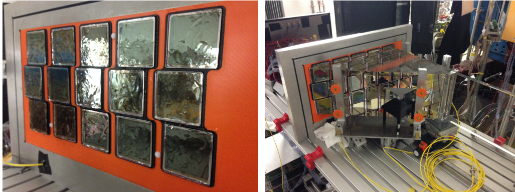
(a) Sensors embedded in plastic matrix with optical grease applied.
