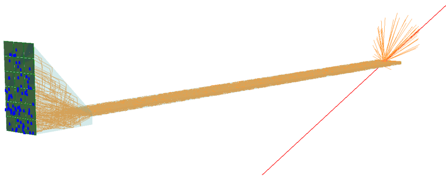
Figure 3.16: Event display of the simulation of a single pion event with \theta = 22^\circ and p = 3.5 \text{ GeV}/c . The geometry contains a single segment of the DIRC barrel. The plate is directly attached to the EV without lens. The pion trajectory is shown in red, the Cherenkov photon trajectory in orange and the hits on the detector plane in blue.
