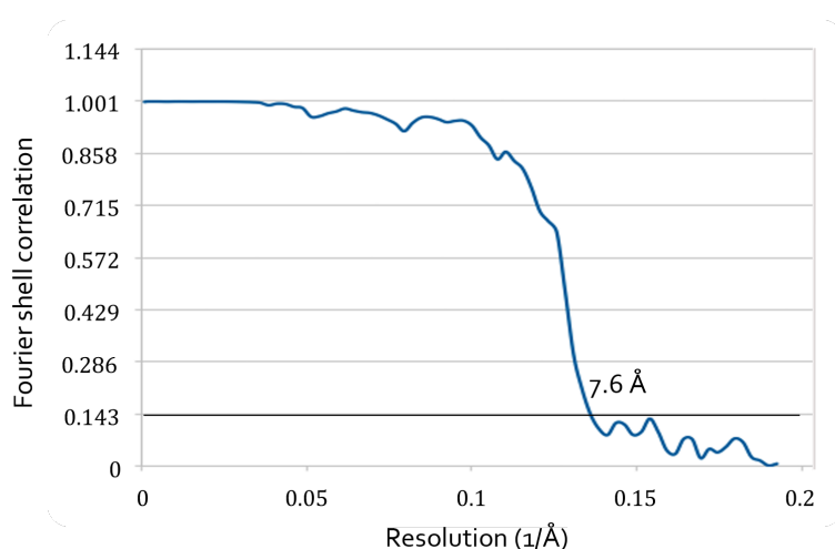
Figure 35 FSC curve of the core reconstruction
