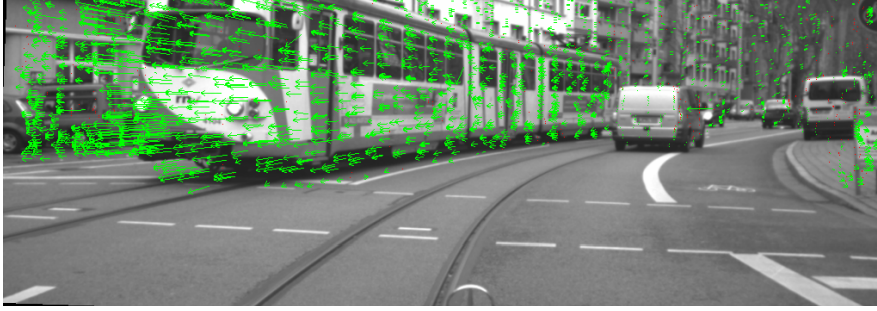
Figure 2.6: Sparse KLT optical flow result based on the ZSSD matching criterion.
