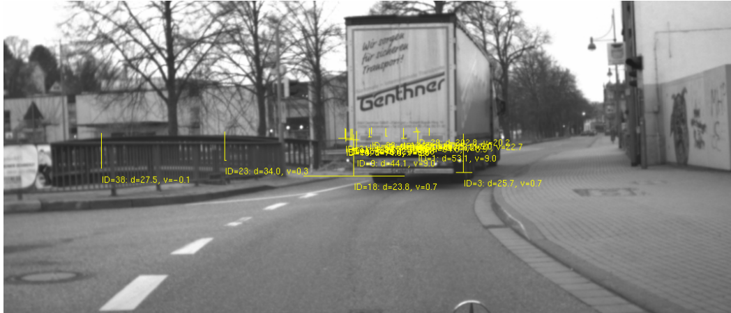
(a) Radar object hypotheses. The Radar object hypotheses marked by flipped, yellow T symbols can define the full parameter vector \Theta_{map} .
