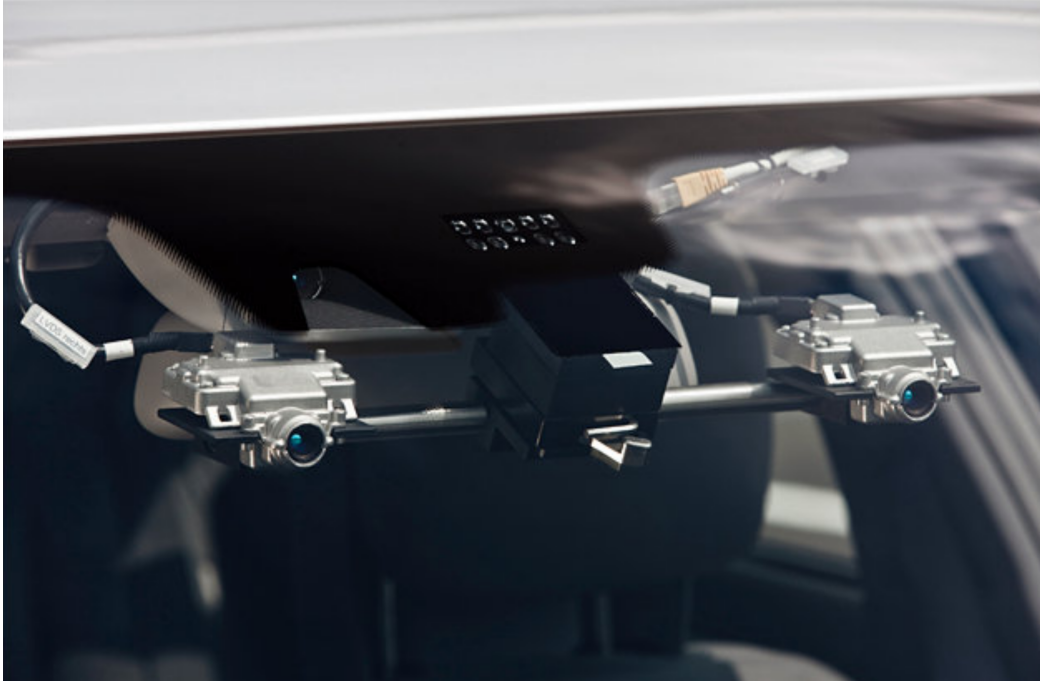
Figure 3.14: Picture of the used stereo camera system mounted behind the windshield of the experimental vehicle. A detailed specification of the cameras is given in the main text.
