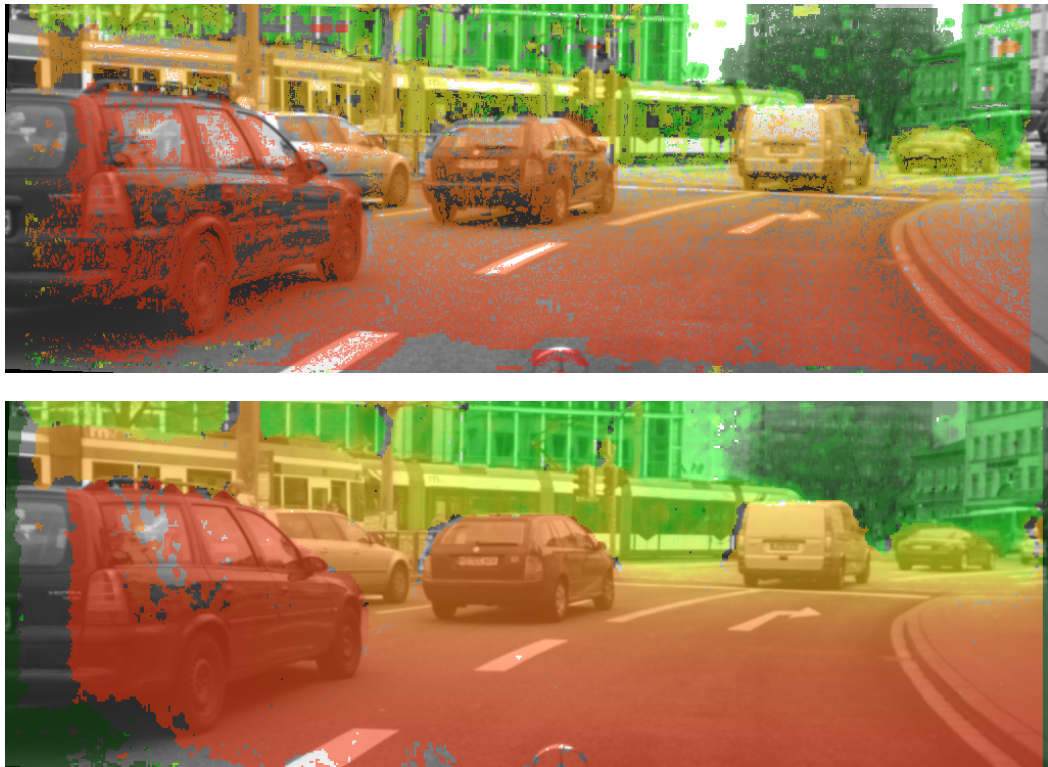
Figure 2.3: Comparison of a sparse correlation-based disparity map shown above and a dense disparity map obtained from SGM below. The sparse correlation stereo is much noisier with clear blob-like reconstruction errors in the upper part of the image, SGM performs significantly better. The color encodes the disparity (red=large, green=small).
