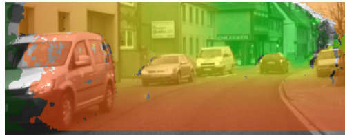
(b) SGM [Gehrig et al., 2009] stereo image. The distance is color encoded ranging from red (close) to green (far away).
