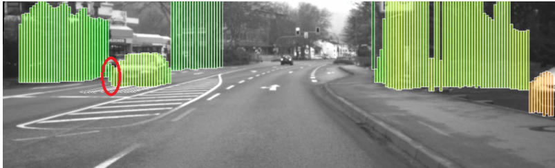
(b) Dynamic Stixel World. The distance is color encoded ranging from red (close) to green (far away). The tear-off edge is marked red.
