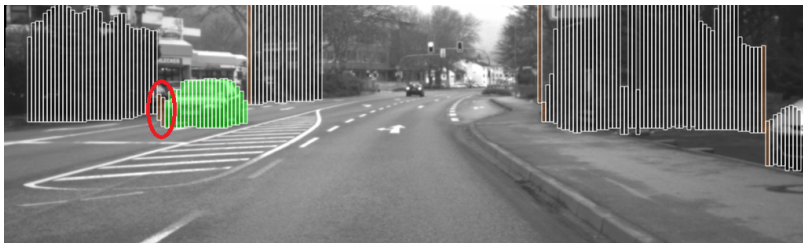
(d) The solution. The phantom Stixels are correctly classified as Out_{\tau}^L outlier Stixels, the corresponding Stixel are marked brown.
