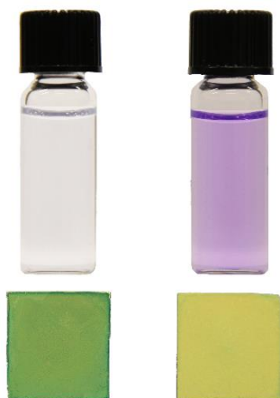
Figure S8.4.4 Color differences of dye selectively loaded PTA@HKUST-1 SURMOFs (left: the SURMOF is selectively loaded with MB after immersion into MB-MV-RhB mixture; right: the SURMOF is selectively loaded with MV after immersion into MV-RhB mixture) after being soaked in 0.025 M \text{NH}_4\text{Cl} ethanol-water solution (the volume ratio of ethanol/water is 160).
