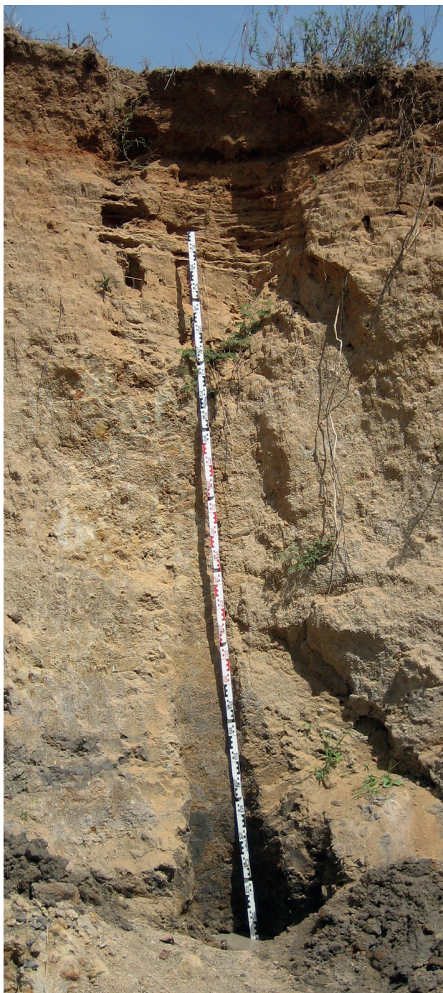
Fig. 5. Soil profile in the Nok Valley with blue-grey clay at the bottom. Length of scale: 3 m. Photo taken in 2009.
