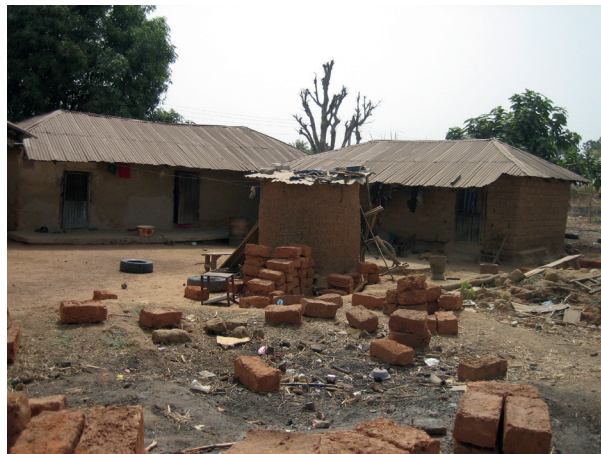
Fig. 30. Mud bricks drying in the sun, in the village of Chinka. Photo taken in 2009.
