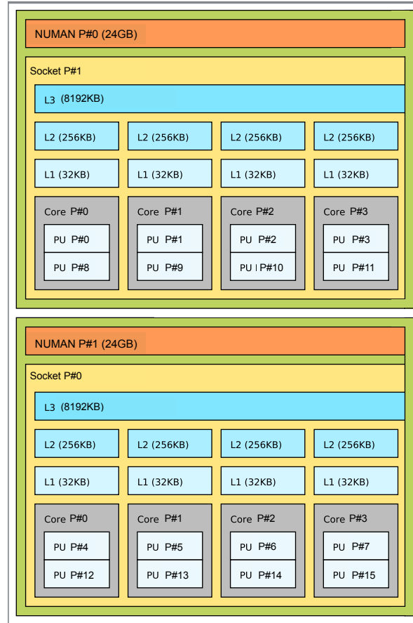
Figure 3.7: The structure of the lxir039 server at GSI, which is equipped with two Intel Xeon X5550 processors. Due to HTT, it can operate in total with 16 threads in parallel. Each core of CPU has 32 KB of L1 cache and 256 KB of L2 cache. 8 MB of L3 cache memory is shared among the cores of a CPU.
