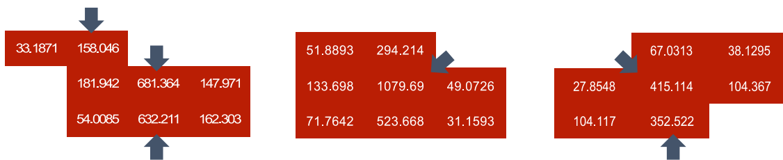
Figure 6.11: Three examples of large clusters measured by the RICH detector. The gray arrows indicate positions of local maxima identified with the Maximum7 search mask. The numbers depict the charge of each pad.
