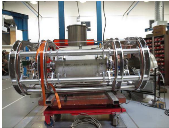
Figure 5. Sc cw-LINAC-demonstrator comprising a CH cavity embedded by two sc solenoids on a support frame, to be mounted inside the cryostat.
