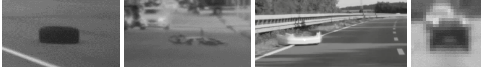
Figure 1.1: The detection and accurate localization of distant and/or small generic obstacles represents a major challenge for perception systems of intelligent vehicles.
