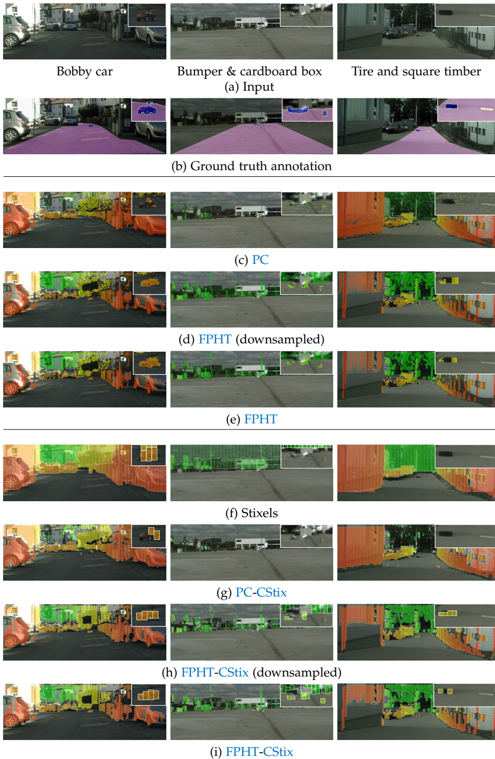
Figure 3.16: Qualitative results of the evaluated methods on the Lost and Found test subset. The top two rows show the left input image and the ground truth annotation, lower rows show pixel-wise and mid-level detections as overlay, color-coded by distance.
