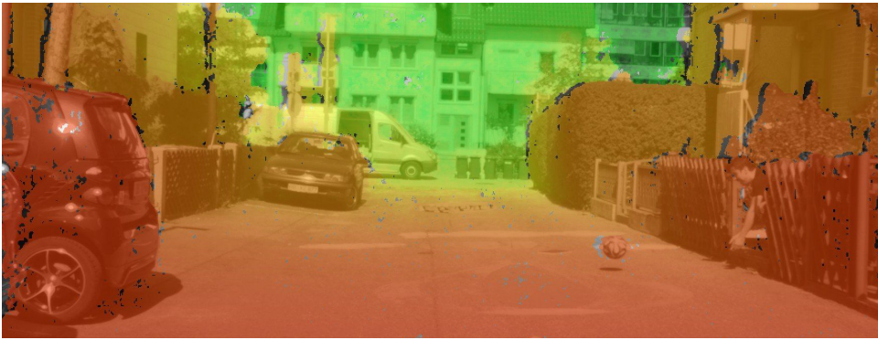
Figure 2.5: Example of a dense disparity map computed via the Semi-Global Matching (SGM) algorithm [Hirschmüller, 2008, Gehrig et al., 2015]. The pixel-wise disparity results are visualized as a color-coded overlay, where green represents small disparity (large distance) and red represents large disparity (small distance).
