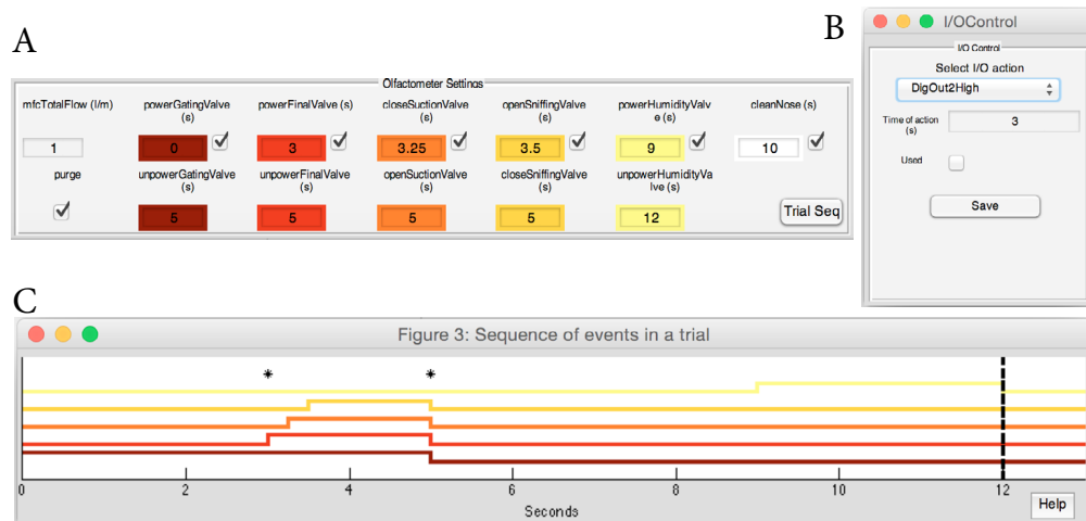
Figure 3.3: A Sequence of events during a typical trial. The GUI allows the user to set the total flow rate of the presented odorant and the times of several valve actions. Writing a vector (multiple numbers surrounded with brackets) in the field results in multiple instances of the valve-opening or closing in one trial at the defined times. Name, number and default values of these valve actions can be defined in configuration files. In this example the times of opening and closing valves gating the odorant, the final valve gating the line to the animal and several custom valves can be set. B Another GUI component allows the user to add I/O actions to the current trial. Available I/O actions enable the user to start real time execution of the sequencer by external triggering and controlling 3 digital output lines. Custom I/O actions can be defined, ranging in complexity from controlling a certain digital trigger to sequences of code allowing closed loop experiments. C The GUI visualizes the sequence of events during one trial. Lines denote the open (high) and closed (low) state of the valve stars denote onset times of digital outputs. The broken line denotes the end of the trial (time of the last action).
