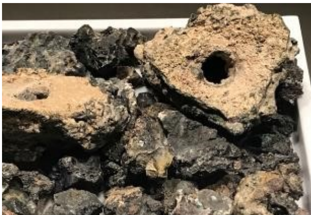
Slag remains provide evidence for the mass smelting of copper at the site. The hole reveals where a pipe was inserted to help to control the temperature in the furnace.
