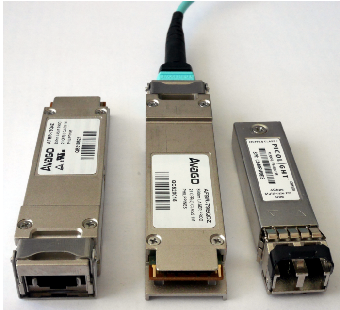
Figure 1.17: Photo of two QSFP modules with four bi-directional links each and one SFP module on the right with one bi-directional link.
