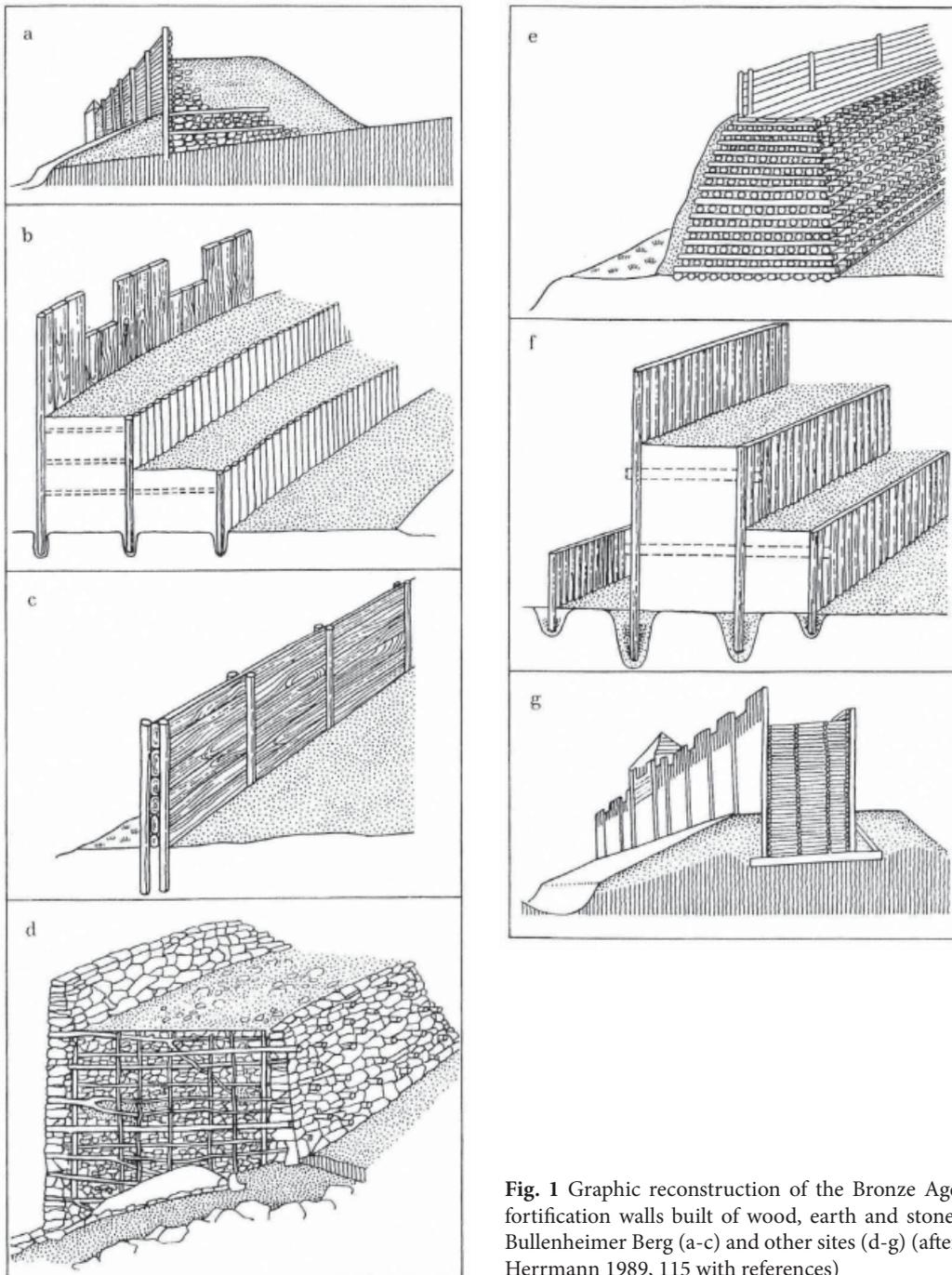
**Fig. 1** Graphic reconstruction of the Bronze Age fortification walls built of wood, earth and stone. Bullenheimer Berg (a-c) and other sites (d-g) (after Herrmann 1989, 115 with references)
