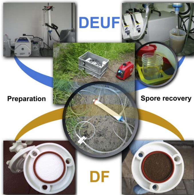
Fig. 2. Water sampling procedure. For the DEUF method (blue) the preparation of the ultrafilter matrix with blocking buffer was carried out prior to filtration. After filtration ultrafilter cartridges were eluted, the eluate recaptured in a vessel, subdivided in 12 \times 50 ml screw-cap tubes and stored at -20^\circ\text{C} until further processing. For the DF method (orange) no pre- and postprocessing steps are necessary. Water filtration in the field with parallel DF and DEUF setup (middle). (For interpretation of the references to colour in this figure legend, the reader is referred to the web version of this article.)
