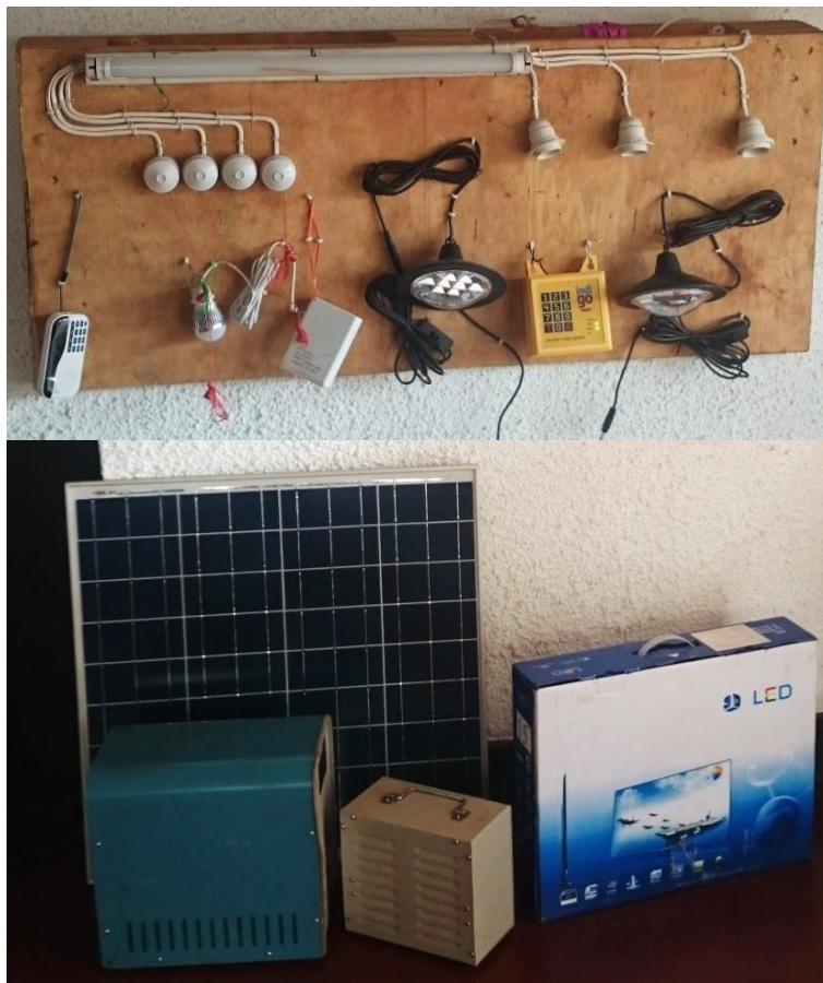
Fig. 5: Presentation-kit for a 80 W solar-home-system
