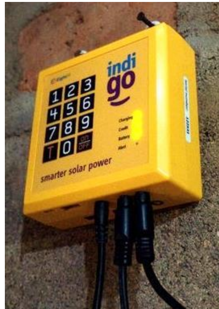
Fig. 8: Off-grid pre-paid meter for SHS
