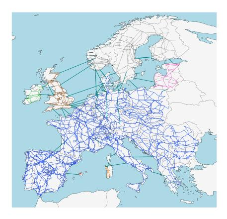
**Figure 3.** The different synchronous zones of the European power system, as indicated by the different colors. Whereas the Continental European grid is the largest subnetwork, Ireland, the United Kingdom, Scandinavia (with only parts of Denmark), and the Baltic region have their own synchronous zones. These areas are interconnected via DC lines (**dark green**).
