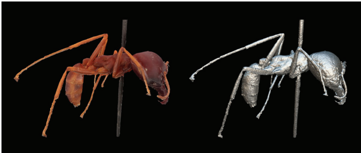
Fig. 3.19. 3D model of a Dorylus ant (size: 1.5 cm) based upon focus stacked images, textured model is on the left, the view of only the mesh is on the right.
