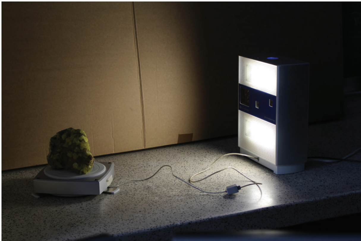
Fig. 3.29. NextEngine with the rotary table holding a geological sample. The cardboard sheet behind is placed to avoid reflection of the bright and shiny glazed white tiles on the wall. The NextEngine also comes with a sample holder to scan small samples.
