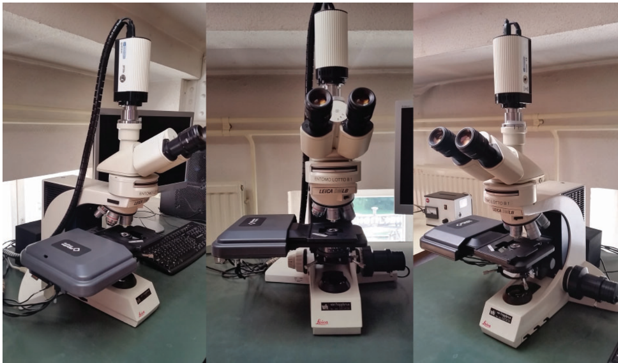
Fig. 2.12. General view of the ‘Information in Images’ system mounted on a Leica microscope at the Royal Museum for Central Africa.
