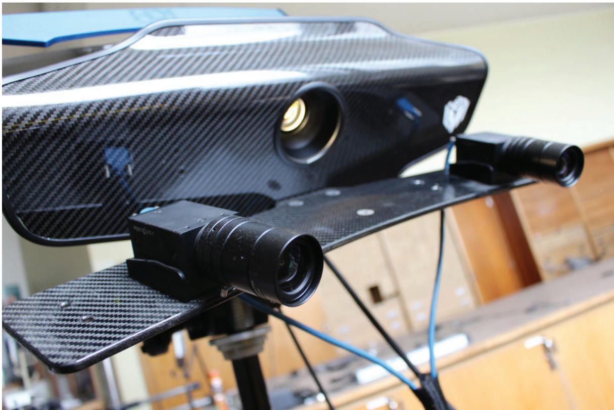
Fig. 3.23. The HDI white light scanner.
