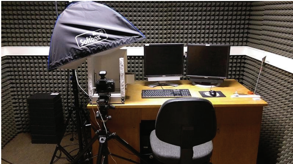
Fig. 2.19. View of the photographic lab of the ZooSphere, with the automated specimen rotator in front of the camera, covered by styrofoam panels to reflect the light in all directions. Image copyright MfN.
