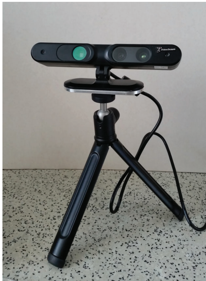
Fig. 3.34. The Primesense infrared depth sensor of the Gotcha with a tripod, allowing it to stand or be used handheld while scanning.
