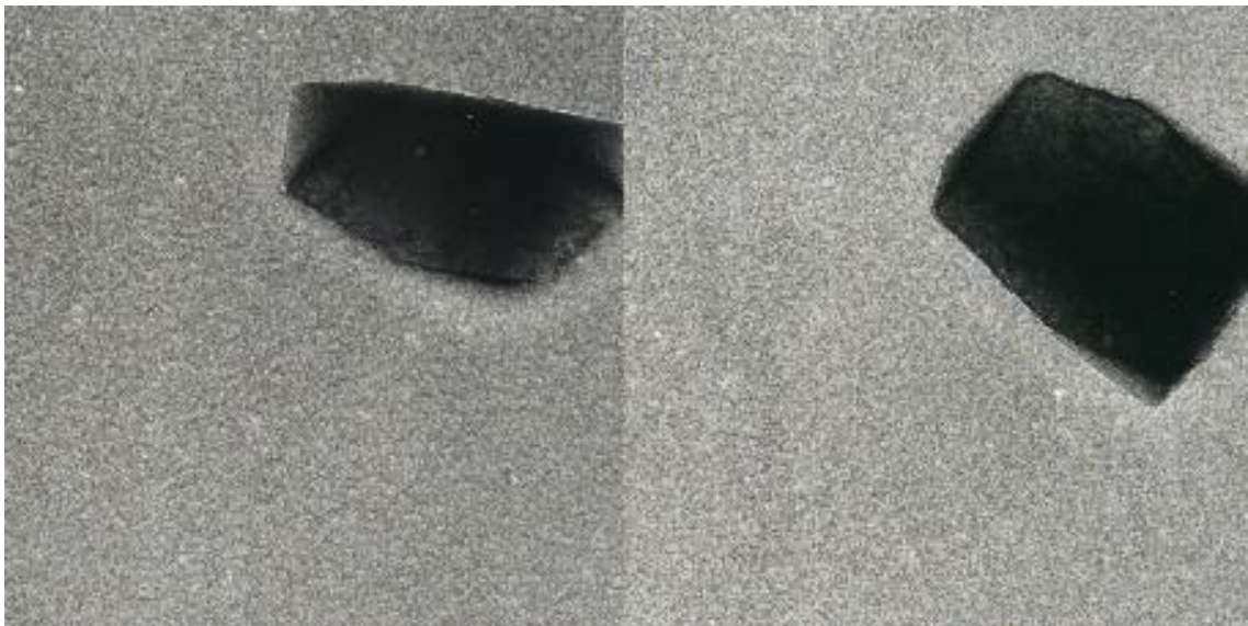
Figure 4.4.3.1.A: GluR-B negatively stained in aurothioglucose at magnification of 46000 \times ; the image on the left side shows the grid tilted by 50^\circ relative to the electron beam. On the right side the same area was imaged in an untilted position. The black contaminant illustrates the effect of tilting.
