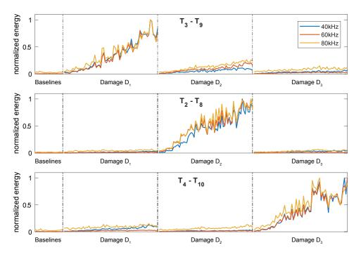
**Figure 11.** Analysis of the normalized signal energy of the differential signal for three representative actuator-sensor pairs (horizontal axis is proportional to an increasing damage size). The normalization was performed using the maximum signal energy for each transducer pair. Damage can be identified best on the straight line between the respective actuator and sensor given by the highest score.
