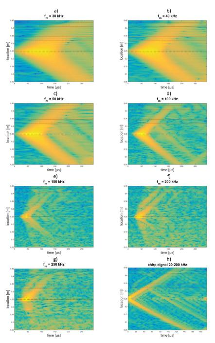
Figure 14. B-Scans of the plate for different excitation signals. Figure (a-g): 5-cycle tone burst for different frequencies, (h): chirp signal. The influence of the stringer can be seen on the upper half space.
