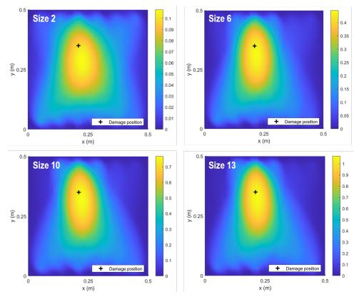
**Figure 12.** Tomographic image reconstruction for damage  $D_1$  and the damage sizes 2, 6, 10 and 13. The peak intensity increases of larger damage sizes as shown by the colorbar. The scaling parameter of the RAPID algorithm was defined here as  $\beta = 1.1$ .
