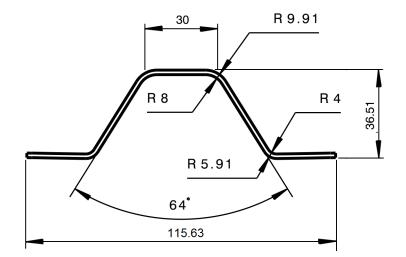
Figure 1. Front view of omega stringer (dimensions in mm).
