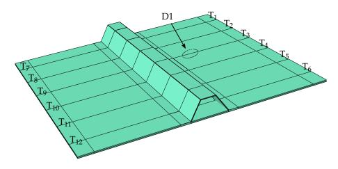
**Figure 16.** Illustration of the finite element shell element modelled in Abaqus. The plate and the stringer are modelled with linear reduced integrated shell elements (S4R) with a seed length of 1 mm.
