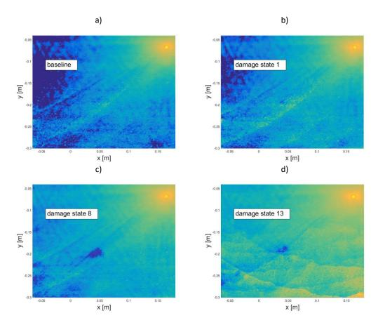
**Figure 15.** (**a**–**d**) RMS-maps of the *wave field plate* with stringer for different damage states. All images are normalized for a better comparability. The yellow spot in the upper right corner is the actuator; the blue spot in the middle represents the damage location.
