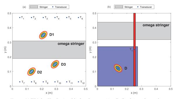
**Figure 3.** (a) *SHM-plate*: Visualization of the three damage positions  $D_1-D_3$  relative to the transducer locations  $T_1-T_{12}$ . Given by the laminate stack the orientation of the reference damages is 45° (b) *Wave field plate*: measurement area for SLDV measurements applying the reference damage (purple) and line scan orthogonal to the stringer element to assess its influence on wave propagation (red).
