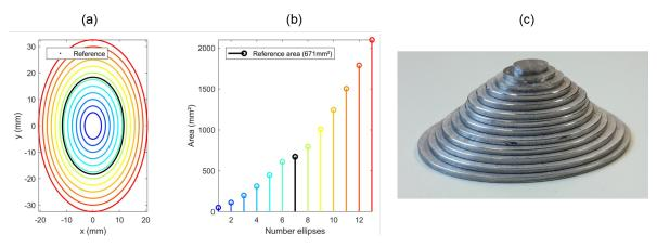
**Figure 5.** (**a**) Geometry of the elliptical reference damage (**b**) Area of the elliptical reference damage (**c**) Fabricated reference damage (steel).
