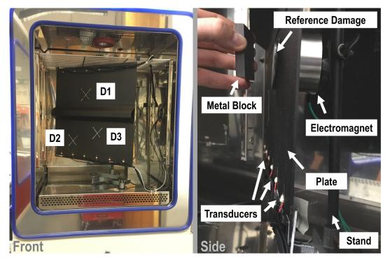
**Figure 6.** Front view of the *SHM plate* in the climate chamber (**left**). Two temperature sensors were installed on the top right and bottom right for surface temperature measurements. Side view (**right**) before the fixation of a reference damage using a metal block and the electromagnet.
