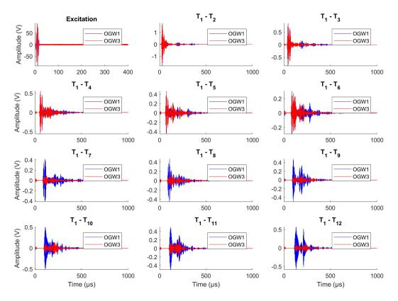
**Figure 9.** Ultrasound measurements at  $f_c = 260$  kHz of the flat *SHM plate* (OGW1) and the *SHM plate* with stringer (OGW3). In this example, the first transducer  $T_1$  works as actuator and all other transducers  $T_2$ – $T_{12}$  serve as receivers. The influence of the stringer can be clearly identified especially for receivers  $T_7$ – $T_{12}$  that are located on the opposite side of the stringer.
