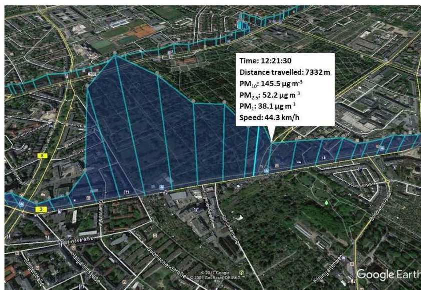
Figure 1. kml file with the local in-cabin particulate matter (PM) concentration measured while driving through Frankfurt am Main. Turquoise line: Location-dependent PM concentration. Geographical picture by Google Earth.
