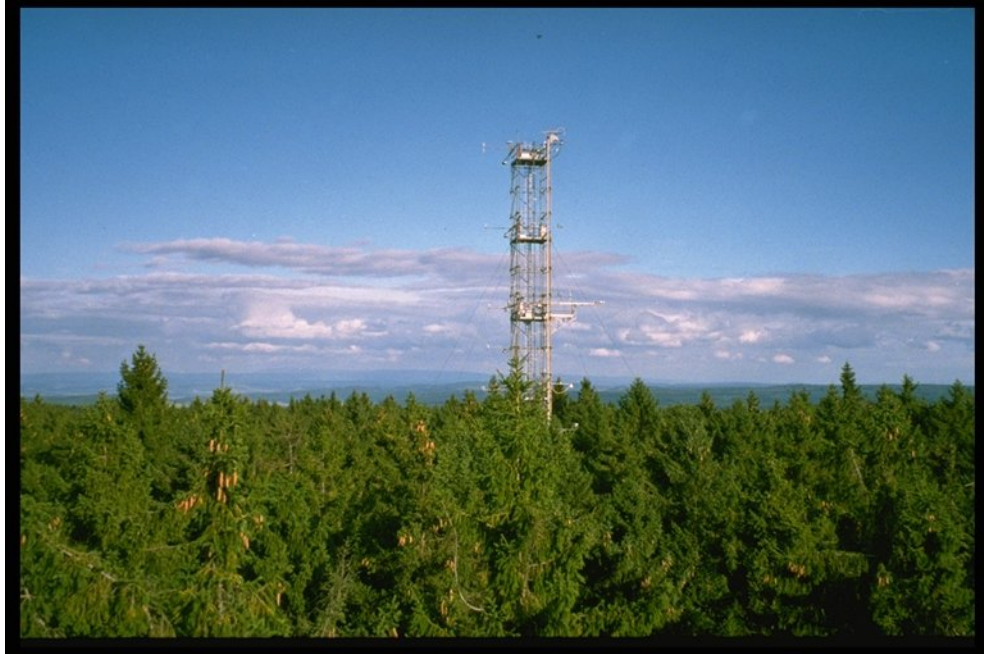
Figure 3.8: The meteorological tower from which air samples for REA measurements were collected. The sonic anemometer-thermometer is mounted at the height of 39 m, which is about 3 m higher than the 3rd platform from the top. (Courtesy: Martin Steinbacher)
