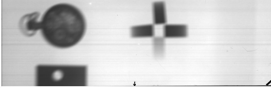
FIGURE 4.34: Image taken by IP with magnifications of M = 2 . The source size of the X-ray tube leads to a washing out of the structures seen.
