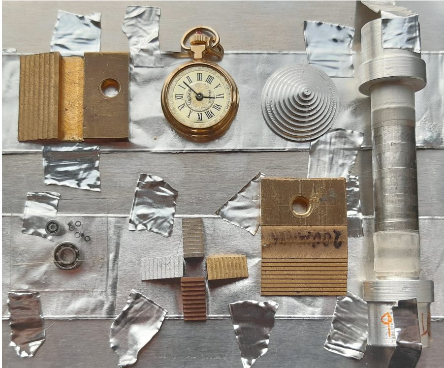
FIGURE 4.30: Picture of the radiography targets used in the experiments. The targets consist of several materials which allows comparison between Al, Cu, Fe and brass (alloy of Cu and Zn). The geometry of the different steps is the same (1 mm each).
