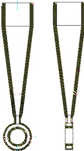
Figure 2.13: Half stems geometry including the water cooling channel.
