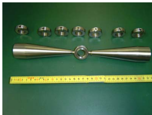
Figure 2.14: View of one stem together with the central rings: it is possible to see the aperture for the cooling water.
