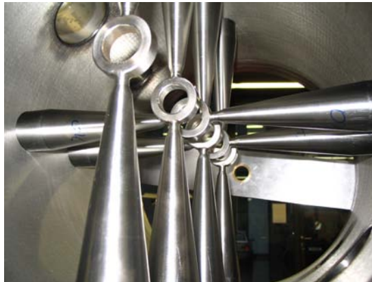
Figure 2.16: The inner part of the cavity after welding.
