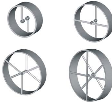
Figure 2.9: The potential H-Mode structure. The number m of stems per drift is responsible for the resonant mode H_{m11} .
