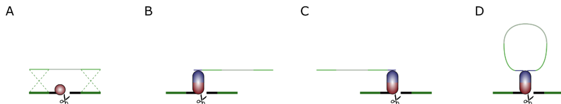
Figure 4.1 – Model of the conformation of the HDR machinery in combination with Cas9 fusions. A The homology arms (green lines) of the targeted site extend to either side of the cut made by Cas9 (red sphere) and the HDR donor is positioned accordingly. B Cas9-N57 or Cas9-N123 recruit the HDR template to the target site via interaction between the N57/N123 domain (blue semicircle) and the 14DR SB binding site in the donor (blue line), positioning the left end of the donor close to the cut site. C Same as B, with the SB binding site on the right end of the donor. D Presence of SB binding sites on both ends of the donor might result in an unfavorable loop formation.
