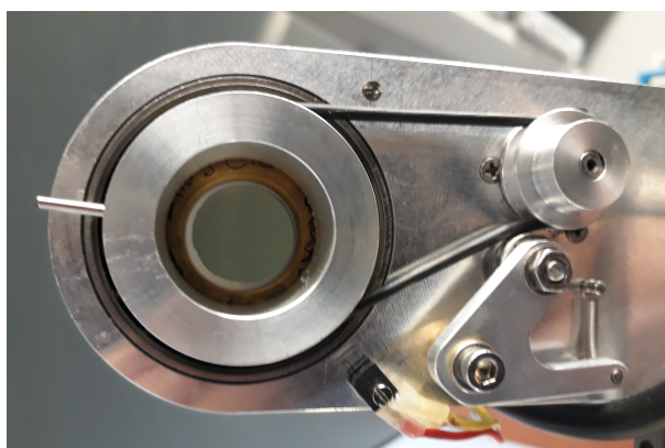
Figure 4.3.2: Rotational sample holder: The sample cell is rotated by a motor via an elastic band (black) while the whole arm is moved upwards and downwards by an additional motor.
