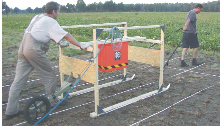
Figure 4.8: Picture of experimental setup to determine the coefficient of reflection: A 1 GHz GSSI horn antenna is mounted on a sledge 0.53 m above the ground.
