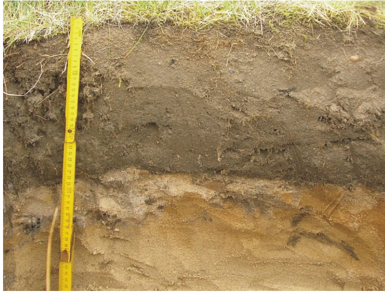
Figure B.1: Picture of soil profile at location 1. Soil horizons due to German soil classification (Ad-hoc-AG Boden, 2005): 0–28 cm: rAp, 28–40 cm: rAp+ Ae+Bs, 40–50+ cm: Cv.
