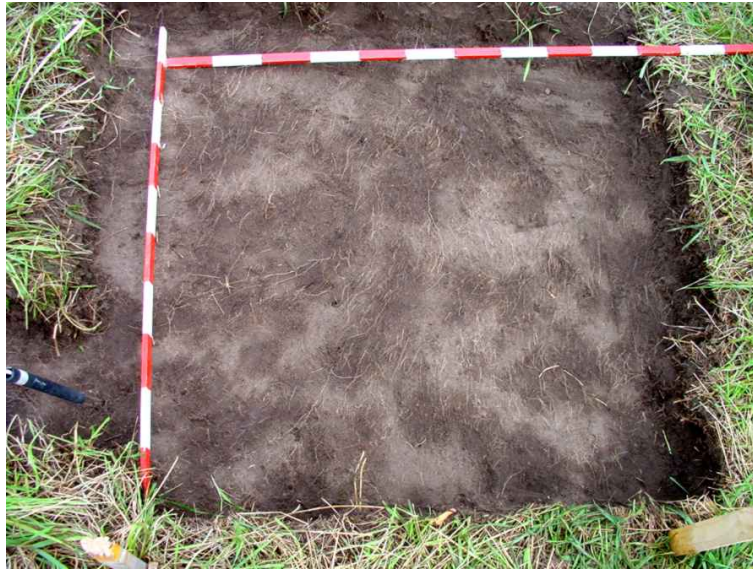
Figure 1.1: Picture of sandy soil demonstrating soil heterogeneity on an area of 1\text{ m} \times 1\text{ m} . The turf has been removed and the pattern corresponds to the soil moisture (dark parts = moist soil, light parts = dry soil), pers. comm. Schmalholz, TU Berlin ( http://www.interurban.de ).
