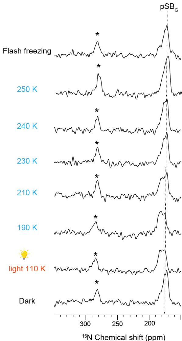
Figure 43: DNP-enhanced ^{15}\text{N} CP spectra of [ ^{13}\text{C}_3 -Retinal, ^{15}\text{N}_z -Lys]-KR2 (100 mM NaCl) in dark state, after illumination at 110 K and relaxed up to 250 K and the sample trapped by flash freezing. * indicates the spinning side bands. There was no deprotonated Schiff base signal (usually around 320 ppm) observed.
