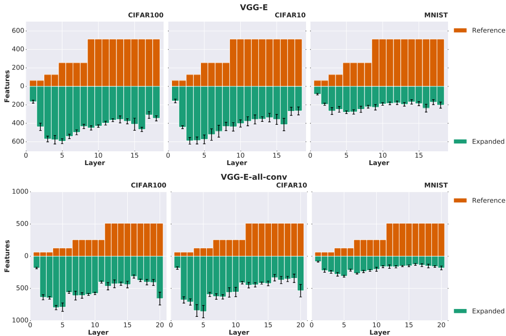
Figure 3: Mean and standard deviation of topologies as evolved from the expansion algorithm for a VGG-E and VGG-E all-convolutional architecture run five times on MNIST, CIFAR10 and CIFAR100 datasets respectively. Top panels show the reference architecture, whereas bottom shows automatically expanded architecture alternatives. Expanded architectures vary in capacity with dataset complexity and topologically differ from their reference counterparts.
