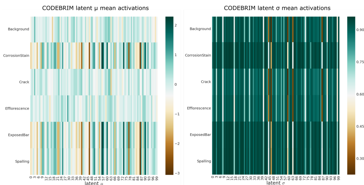
Figure 2.6: 60-dimensional Gaussian mean and standard deviation encodings averaged over the entire CODEBRIM training dataset. It is observable how some defect categories are clearly separable, whereas others have strong distributional overlap and distinction is based on nuances in particular modes. Figure taken from Mundt et al. (2018a).
