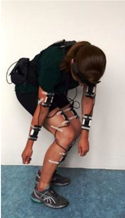
Fig. 1 ▲ Image of the computer-assisted acquisition and long-term analysis of musculoskeletal loads (CUELA; IFA, Sankt Augustin, Germany) measuring system
