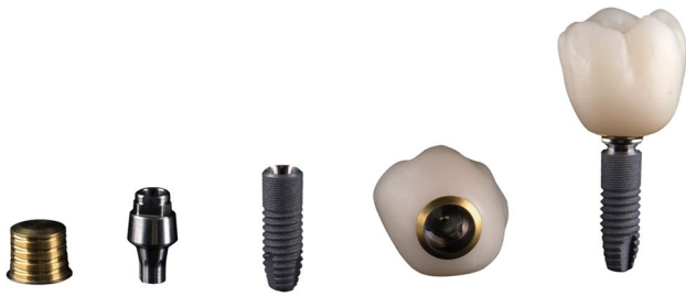
Fig. 1 Components of Acuris conical indexed abutment-system illustrated by the example of Astra Tech EV (from left to right): titanium nitride (TiN) Acuris cap, conical Acuris abutment with anti-rotation connection, implant, extraorally luted all-ceramic crown on TiN cap, conometrically fixed crown-coping complex on assembled abutment
