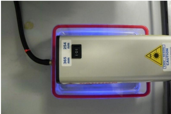
Figure S1: Experimental setup including valve for argon, reaction chamber and UV-lamp.
