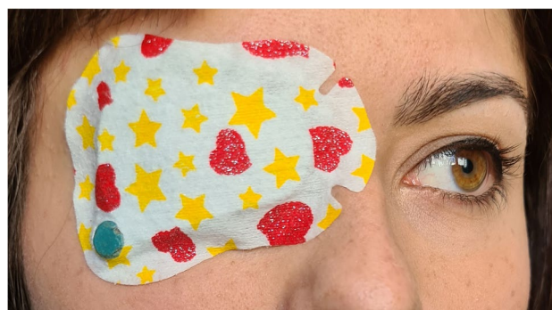
Fig. 1 Occlusion patch with a TheraMon® microsensor ( 9 \times 13 \times 4.5 mm) attached to its inside and visible through a hole made at the lateral inferior margin of the patch. The microsensor measures the environment temperature every 15 min, has a memory capacity of 100 days and a battery life of 2 years
