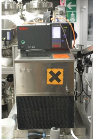
(a) Huber CC-405 cooling thermostat.
