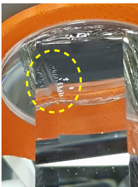
Figure 4.50: A snow flake-like structure can be seen on the bar-lens joint.
