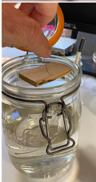
Fig. 10 Prepared specimen to be placed in acetone bath.
