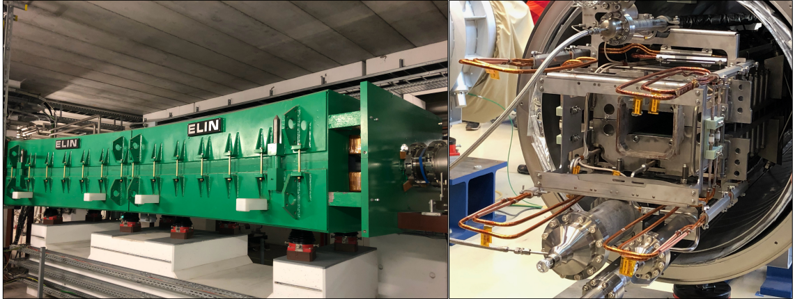
Figure 2.5.: Examples of sector magnets. (left: 7.5° bending dipole of the GSI fragment separator FRS, right: 3.3° super conducting dipole of the SIS100 synchrotron)
